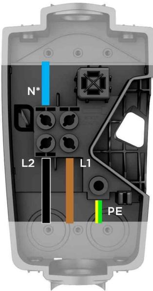
\*When connecting to a 230 V delta no neutral grid, land one of the line connections in the neutral terminal of the wirebox.
